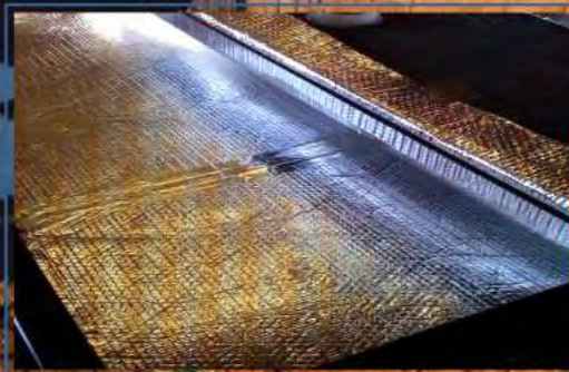
R-15 Astro-Foil Roof, Slide-Out Floor, Entire Underbelly, Additional Wrap Around Holding Tanks
