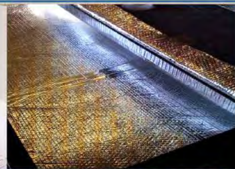
R-15 Astro-Foil Roof, Slide-Out Floor, Entire Underbelly, Additional Wrap Around Holding Tanks
