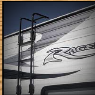
RETRACTABLE ROOF LADDER
