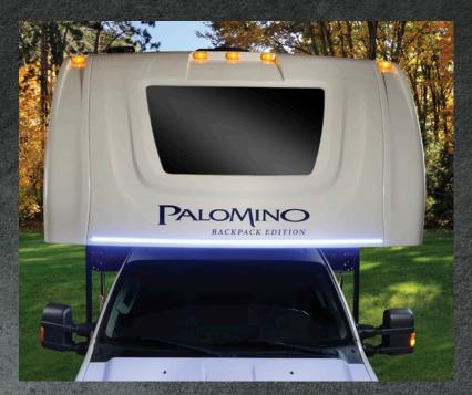
Introducing the Industry First Gel-Coat Fiberglass front cap with a fully integrated windshield. Palomino RV partnered with the leaders in O.E. Automotive Windshield Manufacturing Guardian Industries as well as Dow Chemicals to create this Palomino Exclusive Feature. This automotive style windshield not only looks great rolling down the road, but also creates an open inviting environment in the Palomino Hard Side Max Cabover Bunks while you enjoy great panoramic views.
