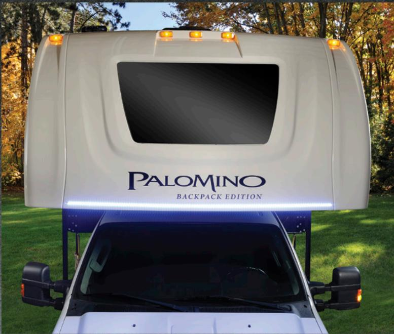
Introducing the Industry First Gel-Coat Fiberglass front cap with a fully integrated windshield. Palomino RV partnered with the leaders in O.E. Automotive Windshield Manufacturing Guardian Industries as well as Dow Chemicals to create this Palomino Exclusive Feature. This automotive style windshield not only looks great rolling down the road, but also creates an open inviting environment in the Palomino Hard Side Max Cabover Bunks while you enjoy great panoramic views.
