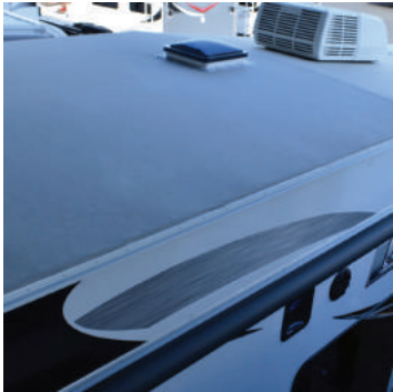
One Piece TPO Roof is energy star rated, easy to maintain and allows us to install vents that clamp into place eliminating screws, reducing potential for leaks. Lance TPO roofs also feature a 12 year limited product warranty.
