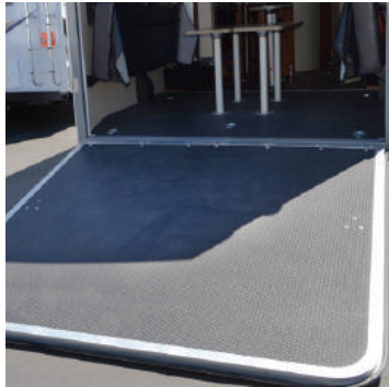
7'2" Ramp Door with Industrial Grade Coin Flooring and Dovetail Floor combine to make loading and unloading vehicles with low ground clearance easier.
