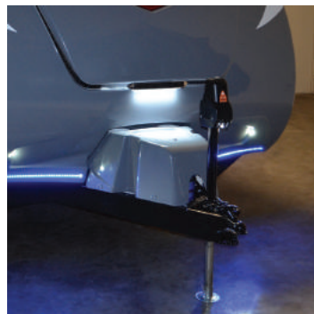
Electric Tongue Jack makes raising and lowering the tongue of your trailer as easy as pushing a button.
