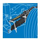
1. Hellwig® helper springs work with the chassis' existing springs to give the RV more support, improving sway control under heavy loads
