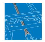
3. Computer-balanced driveshaft ensures reduced shudder and vibrations, and efficient power transfer to the wheels
