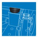
2. Rubber isolation body mounts are positioned near the tires to absorb road shock, dampen noise and minimize vibrations
