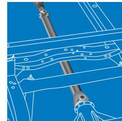
**3. Computer-balanced driveshaft** ensures reduced shudder and vibrations, and efficient power transfer to the wheels
