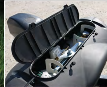
Twin LP Tanks with ABS Cover and Quick-Access Opening
