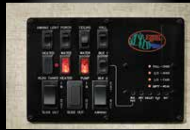
SIERRA's control center allows you to monitor tanks and other systems quickly and easily.
