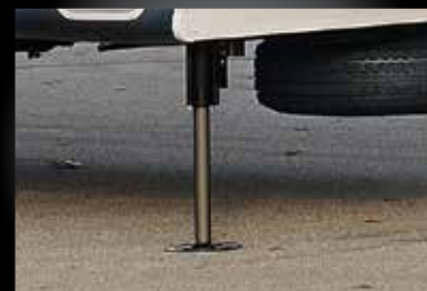
Optional wide stance hydraulic landing gear.
