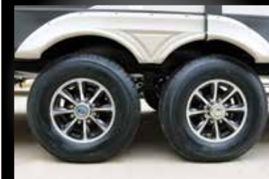
Contemporary aluminum rims with E-rated radial tires. Most SIERRA's feature 7000 Lb. axles.
