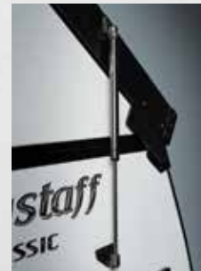
Gas Strut Lift Assist (Std. Hard Side Models w/ Manual Lift Roof Only)
