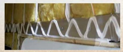
Thick Silaprene super adhesive (475 PSI) quarantees solid contact between the True bonded gelcoat and aluminum frame without lamination
