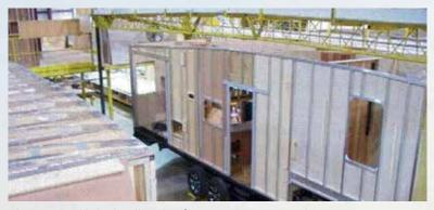
Aluminum studded sidewalls and roof trusses on 16" centers or less
