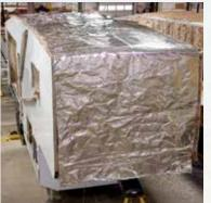
R-38 Radiant shield Therma-foil wrap through ceilings, underbellies and under front cap.
