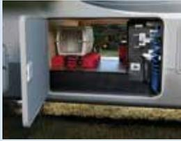
Silverback's front storage compartment is insulated with 1-1/4" thick baggage doors. The central docking station
