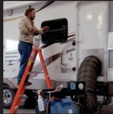
Seal Tech Air Pressure Test
