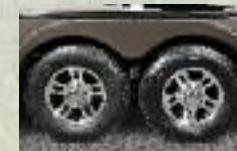
Premium Goodyear® E-rated tires are standard on all models with 8-lug, easy lube axles and aluminum alloy wheels.
