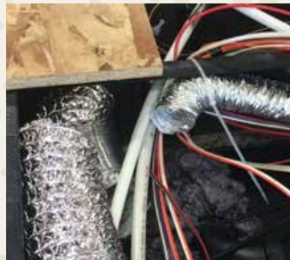
Heated ductwork in the enclosed underbelly helps keep important things from freezing when you need them the most.
