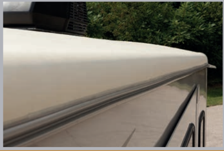
Rolled Edge Roof Line Prevents Pooling And Leaking.
