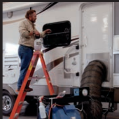
Seal Tech Air Pressure Test
