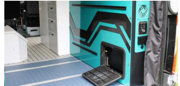
8.4 kWh 51V Lithionics® Power System
