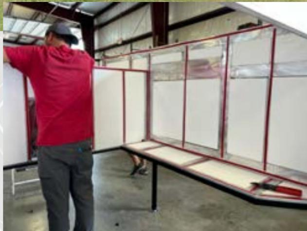
Now with models to fit just about every truck bed size, the OV-X by Soaring Eagle Campers is fully insulated with thick, block foam insulation and covered inside with a composite board, and outside with durable metal sheeting. The roof is strong enough to walk on (in the down position) with strong tubular aluminum framing; is fully insulated; and is covered inside and out with one-piece, seamless fiberglass making it the strongest, most durable roof in the truck topper market.
