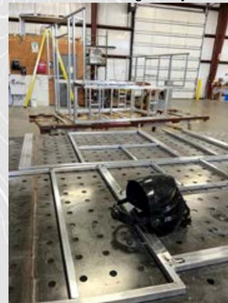
The entire structure of a Soaring Eagle Camper is welded together to form a strong, UNI-BODY construction that
