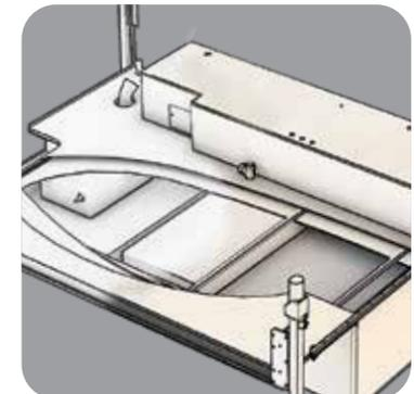
Black Tank Flush. Connect an exterior hose to rinse, flush and clean your tank after use.
