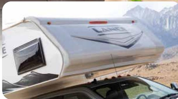
**TPO one-piece front nose cap** is the first line of defense against wind and water intrusion, borrowed from automotive bumper design is sleek and cannot delaminate unlike wrapped fiberglass noses.
