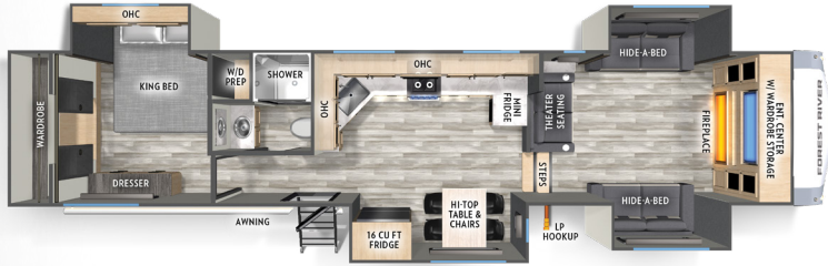
35FL *HITCH: 2,115 *GVWR: 14,115 *UVW: 10,708 CCC: 3,407 **LENGTH: 43' 5" EXT. HEIGHT: 13' 2" *WIDTH: 96" †TANKS (F/B/G): 60 38 76 AWNING: 13'
