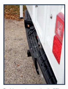
Truck bumper is exposed on the 6'6" short-bed trucks allowing for ease of hitching trailers. 12v lead from all Northstars comes out the rear to conveniently plug into existing plug on truck.
