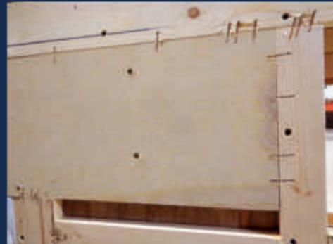
Every Northstar is screwed together at every single joint. Cabinets screwed in from the outside through the wall and also screwed together on the inside. Exterior plywood and low formaldehyde emission paneling make for superior strength & breathability. Northstars are made to last a long time and endure many miles and off road use. It's the Northstar way!
