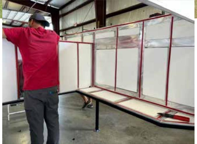
Now with models to fit just about every truck bed size, the OV-X by Soaring Eagle Campers is fully insulated with thick, block foam insulation and covered inside with a composite board, and outside with durable metal sheeting. The roof is strong enough to walk on (in the down position) with strong tubular aluminum framing; is fully insulated; and is covered inside and out with one-piece, seamless fiberglass making it the strongest, most durable roof in the industry.
