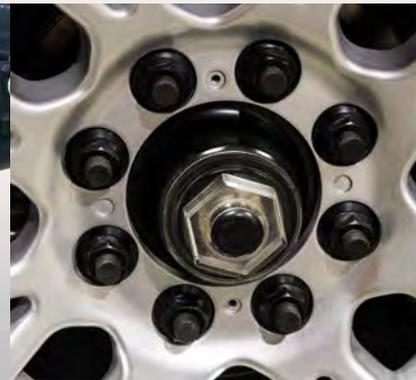
Commercial E-Z Lube® hubs surrounded by 8 large 5/8" stud bolts and standard automotive disc brakes round out the safety features of every DRV unit.
