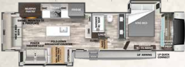
360RL HITCH WEIGHT-2,525 lb. / GVWR-16,525 lb. / UVW-13,134 lb. CCC-3,391 lb. / LENGTH-40' 7" / HEIGHT-13' 5" / WIDTH-96"
