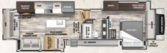
380RL HITCH WEIGHT-2,790 lb. / GVWR-18,000 lb. / UVW-14,389 lb. CCC-3,611 lb. / LENGTH-42' 10" / HEIGHT-13' 5" / WIDTH-96"
