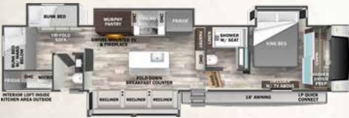
375BHO HITCH WEIGHT-2,430 lb. / GVWR-16,430 lb. / UVW-14,209 lb. CCC-2,221 lb. / LENGTH-43' 1" / HEIGHT-13' 5" / WIDTH-96"
