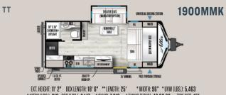
\*HITCH (LBS.): 610 CCC (LBS.): 2,147 \*GVWR: 7,610 ‡ TANKS (F/B/G): 46 30 30 TIRE SIZE: 15"
