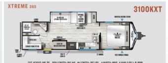
EXT. HEIGHT: 12' 7" BOX LENGTH: 31' 11" \*\* LENGTH: 35' 6" \* WIDTH: 101" \* UVW (LBS.): 8,830 \*HITCH (LBS.); 1,205 CCC (LBS.); 2,537 \* GVWR; 11,405 ‡ TANKS (F/B/G); 53 30 90 TIRE SIZE; 15"
