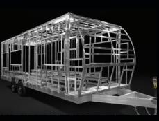
PLĀ<sup>\*</sup> toy haulers are built to last with a fully integrated aluminum frame. The six-sided "welded box" has no fasteners to loosen over time and features a one-piece aluminum roof. Unlike most other toy haulers, there is no wood in our construction to rot and deteriorate over time. PLĀ toy
