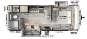
LENGTH: 25' 11" WIDTH: 8' HEIGHT: 10' 11" HITCH: 615 AXLE: 5100 UVW: 5774 CCC: 1841 6 54 GAL 6 60 GAL B 30 GAL
