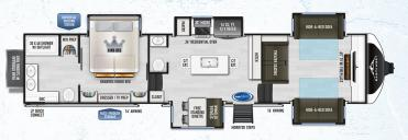
HITCH (LBS.): 3,190 UVW (LBS.): 14,559 CCC (LBS.): 2,631 LENGTH: 41'7" Exterior Height: 13'6" width: 102" tanks [Fig/R]: 64 / 88 / 88 Awning: 16'&14' 380FL
