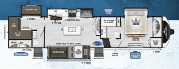
HITCH (LBS.): 2,605 UVW (LBS.): 14,109 GCC (LBS.): 2,496 LENGTH: 41'5" EXTERIOR HEIGHT: 13'6" WIDTH: 102" TANKS 16/6/0; 64 / 88 / 88 AVVINO: 16' & 10'6'
