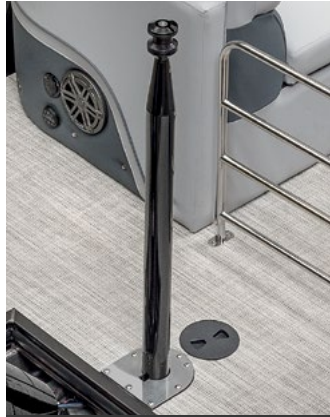
SKI TOW PYLON (Not available on twin engine models)
