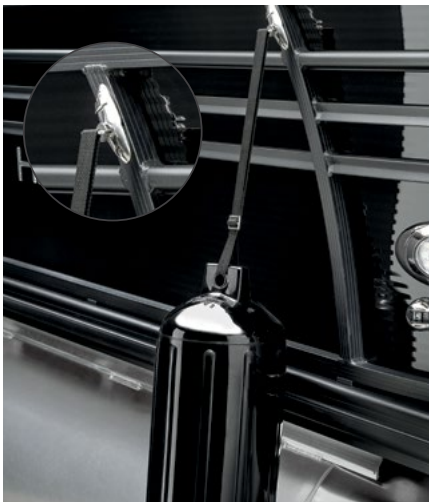
QUICK RELEASE FENDER SYSTEM (Mid-ship quick release available on Solstice, Grand Mariner and Crowne)
