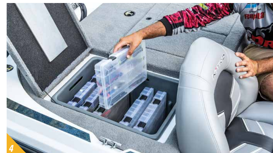
4. 2 lift-out, molded aft storage boxes that will each accept seven 3700 tackle trays
