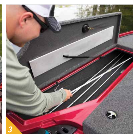
3. Oversized, lockable bow port & starboard rod lockers w/lift assists for rods up to 8'
