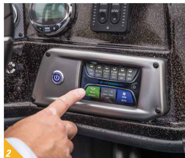
1. Attwood® Centric X folding molded fishing seat w/hydraulic pedestal 2. Touchscreen switch panel w/1-touch boat controls including First Fish, Nite Mode, lighting, bilge, livewells & more 3. Deep V NVT™ performance hull w/RAPID PLANING SYSTEM™ (RPS™) transom
