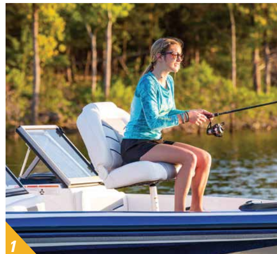
1. 2 convertible & removable fishing seats 2. Aft 16-gal. rotomolded & aerated livewell w/timer, pump-out system & rounded corners 3. Aft swim platforms w/starboard boarding ladder & removable ski tow pylon
