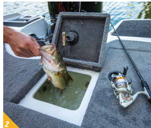
1. 2 convertible & removable fishing seats 2. Aft 16-gal. rotomolded & aerated livewell w/timer, pump-out system & rounded corners 3. Aft swim platforms w/starboard boarding ladder & removable ski tow pylon
