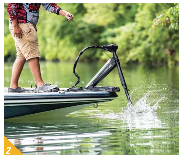
1. Driver & passenger bucket seats w/molded-in, gelcoated storage below each 2. Minn Kota® Edge® 12V, 55-lb. thrust, 45" shaft foot-control trolling motor 3. Custom-molded modular console w/2-tone gelcoat w/Lowrance® HOOK² 4x fishfinder
