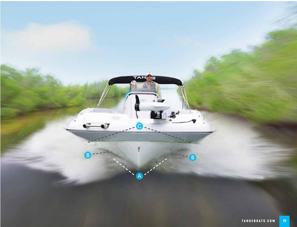
🛕 Deep V hull B HYDROSTEP lifting strakes **C** Reverse chines
