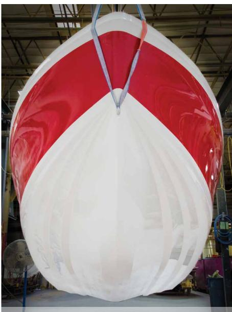
Perfectly prepared molds and careful gelcoat application create a mirror-like shine
