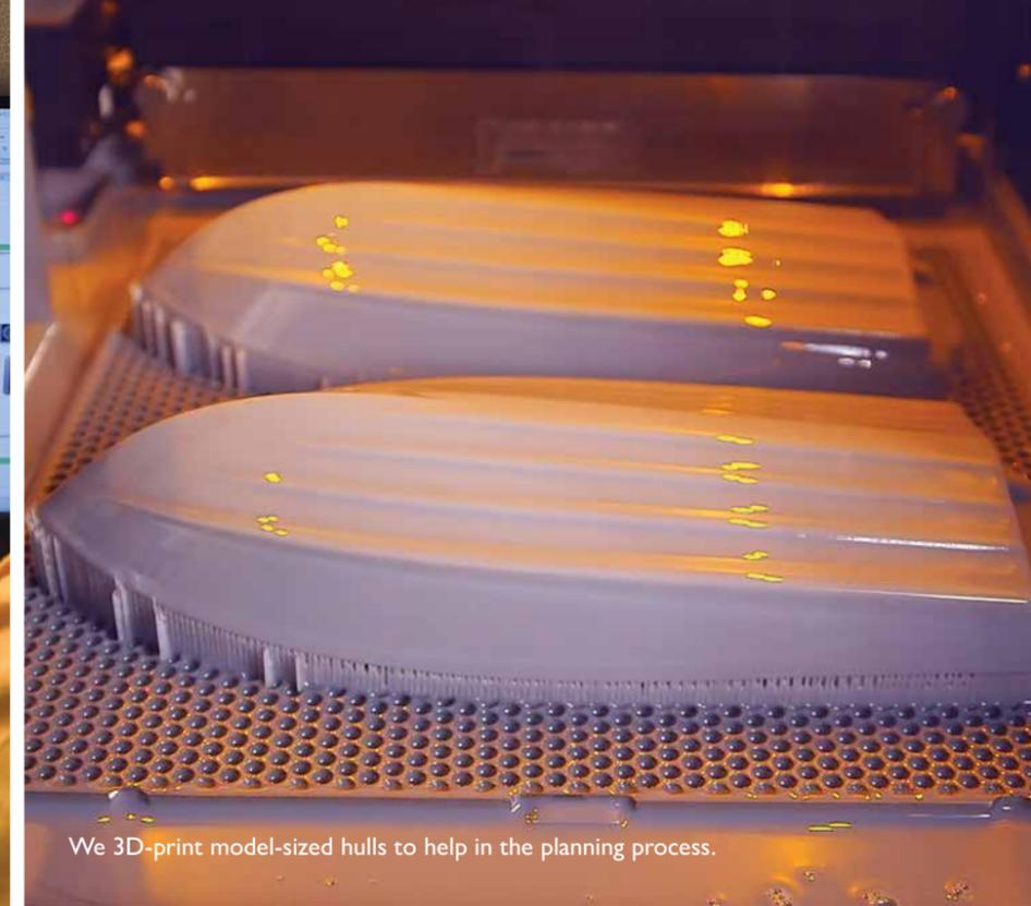
We 3D-print model-sized hulls to help in the planning process.
