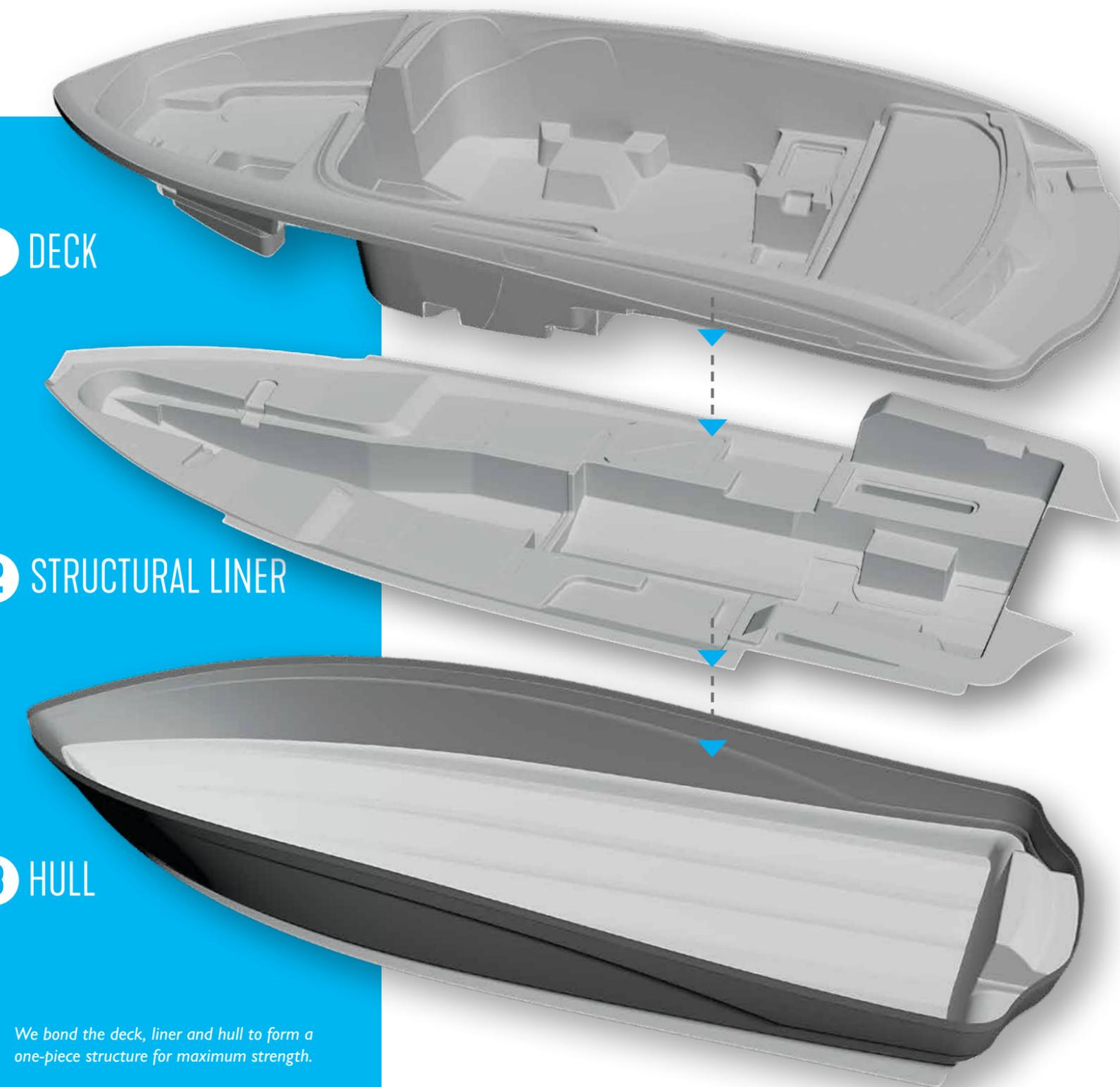
We bond the deck, liner and hull to form a one-piece structure for maximum strength.
