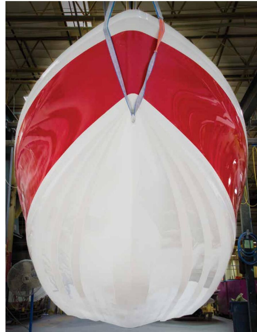
Perfectly prepared molds and careful gelcoat application create a mirror-like shine.
