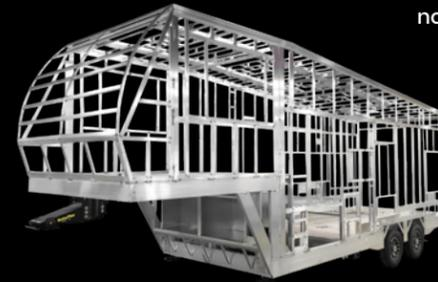
**BUILT TO LAST.** We're called The Aluminum Trailer Company for good reason. Our toy haulers are constructed with a fully integrated aluminum frame. Unlike most other toy haulers, there is no wood in our construction to rot and deteriorate over time. Its six-sided "welded box" has no fasteners to loosen over time and features a one-piece aluminum roof.
