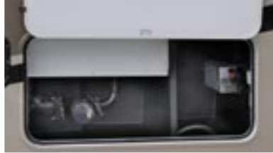
Heated/enclosed holding tanks use warm air from the furnace to protect tanks and valves. (N/A 2251SLE, 2551DSLE, MBS and Transit)
