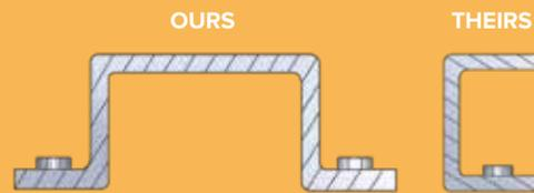
**CROSS CHANNEL CONSTRUCTION:** Provides superior chassis strength. The transom area is supported with up to 3/16" hat-channel construction using twice the amount of fasteners as other pontoons. This provides the strength needed to handle the high torque of today's large engines.
