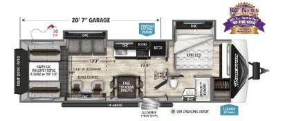
30**G** UVW HITCH GVWR LENGTH HEIGHT CAPACITY 20'7' GARAGE 8,800 1,350 13,000 34'11" 12'4" 100 78 39
