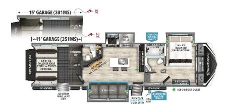
UVW HITCH GWVR LENGTH-HEIGHT CAPACITY 351**MS** 13,800 2,785 16,800 38'6" 13'5" 155 78 78 11' GARAGE UVW нітсн GWVR LENGTH HEIGHT CAPACITY 381**MS** 14,700 2,800 20,000 42'9" 13'5" 155 78 78 15' GARAGE
