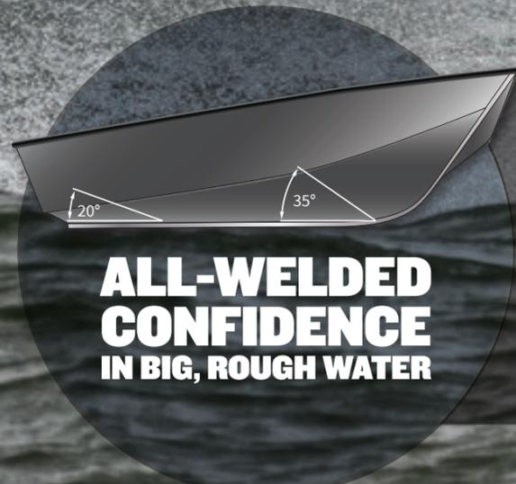
Heavy-duty marine-grade aluminum is joined with welded seams for unmatched strength. A 35° angle at the bow cuts through waves and reverse chines deflect water downward for a dry, smooth ride in rough water.
