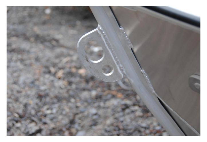
Check out our competitors bolted in bow eye adding additional holes in your hull. Marlon's are welded with an additional hole for your trailer safety chain!
