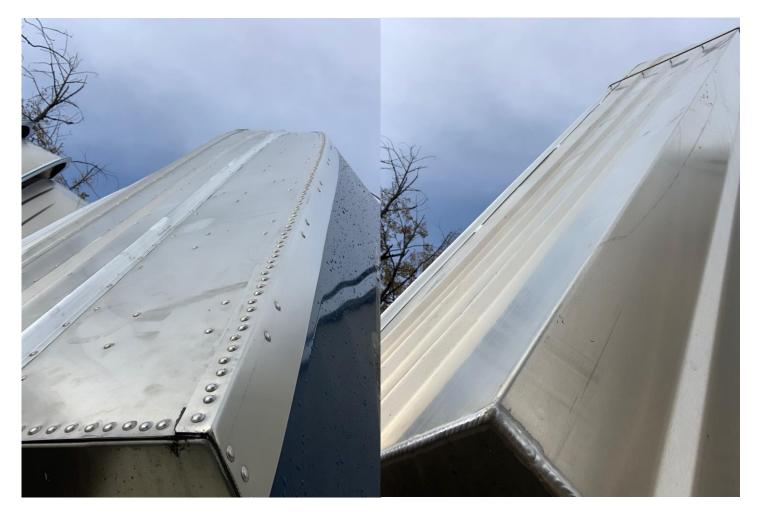
We lost count on how many holes are placed in the sides and transom of most boats in this size category. There is 148 in the transom alone on this competitive boat shown on the left! Our sides are a one piece continuation of the bottom and our transom is sealed with a weld shown on the right.
