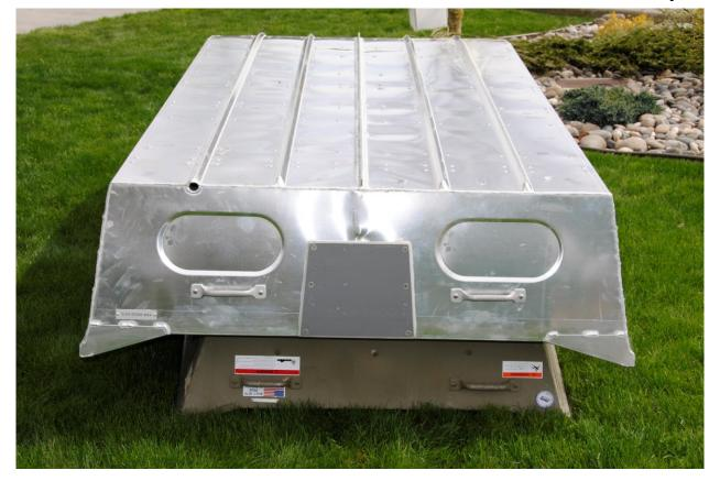
Our wide chine bottom & gunwale equals more carrying capacity 434 lbs vs 200 lbs, more stability and on plane faster with less HP 10' first designed to fit between the wheel wells of a full size truck.
