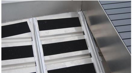
Riveted bow cap removed – replaced with welded bow
