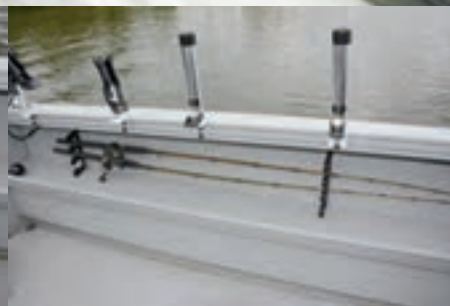
OPEN ROD STORAGE AND INTEGRATED GUNNEL TRACK SYSTEM WITH OPTIONAL BERT'S CUSTOM TACKLE ACCESSORIES
