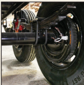
7K DEXTER EX LUBE AXLES WITH NEVR-ADJUST BRAKES
