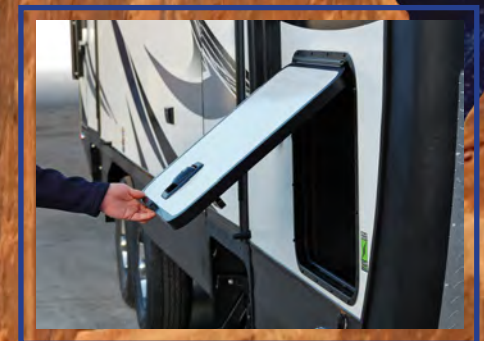
1" Thick Thermal Insulated Luggage Door Compartments
