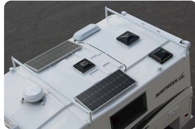
Boat Rack and Dual Solar Panels
