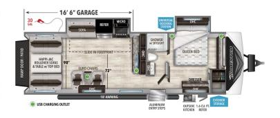
28**G** UVW<sup>1</sup> HITCH<sup>1</sup> GVWR LENGTH<sup>1</sup> HEIGHT CAPACITY 16'6"GARAGE 8,500 1,300 13,000 33'11" 12'4" 100 78 39
