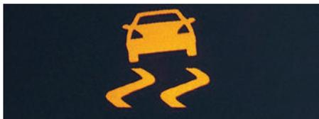
**LOAD-ADAPTIVE ELECTRONIC STABILITY PROGRAM (ESP®)** This dynamic handling system actively intervenes to help keep the van firmly under control and safe by automatically braking individual wheels and reducing engine power to help stabilize the vehicle if wheelspin, understeer, or oversteer is detected.
