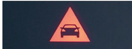
**ACTIVE BRAKE ASSIST** This advanced system senses the likelihood of a collision with a vehicle ahead and sends both a visual and audible warning followed by initiating autonomous braking.
