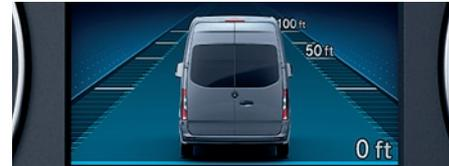
**ACTIVE DISTANCE ASSIST DISTRONIC®** This intelligent cruise control system senses traffic conditions and actively controls your speed to keep you at a safe distance.
