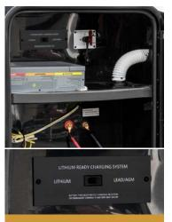
Durango's standard LITHIUM-READY CHARGING STATION includes a dual converter, which allows you to choose between lithium or lead batteries with a flip of a switch!
