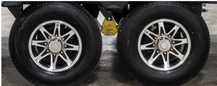
**ALUMINUM WHEELS** 8-lug heavy-duty aluminum rims with 16-inch G-range radial tires
