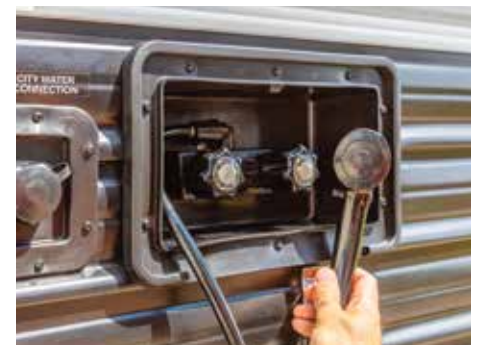
Outside Shower with Hot & Cold Water
